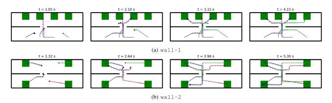
Fig. 2. Benchmarks and results. Dashed-lines are the PWL paths found by the proposed method; Solid lines are the actual trajectories tracking the PWL paths. For each benchmark, we show four snapshots of the simulation with a clock in the title. The dots indicate the current locations of the agents, and agents are marked in different colors.
